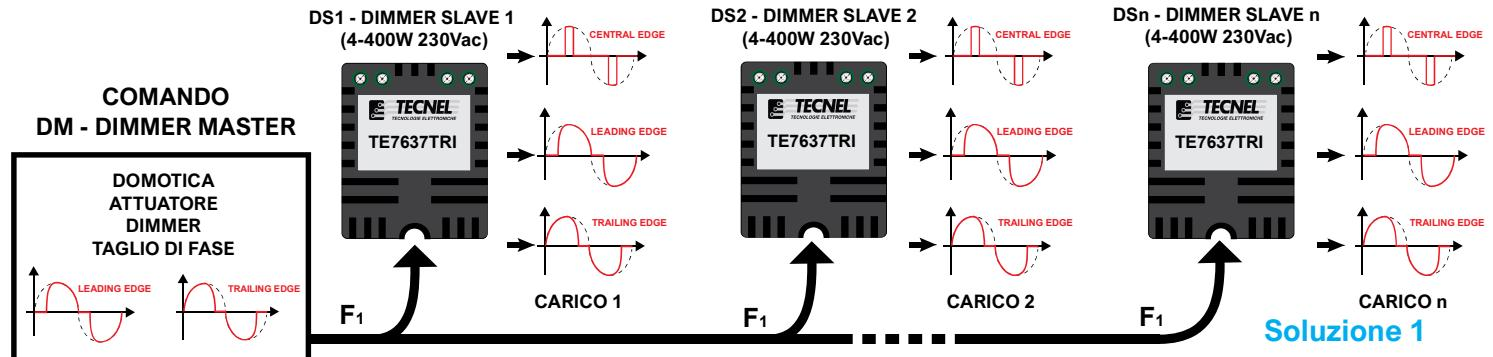
**codice TE7637TRI SCHEMA DI COLLEGAMENTO PROGRAMMATO IN CENTRAL EDGE 4-400W 230Vac**
